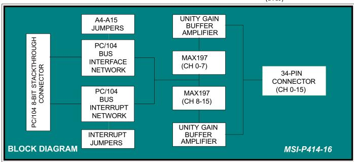
of each channel into a 12-bit digital signal. Low span and offset errors result in no adjustments being required for these functions. Typical total conversion times of 12 us gives a sample rate of 83 ksps for each group of eight channels yielding rates up to 166 ksps for 16 input channels.
