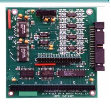
±5V and ±10V with a linearity of 1/2 LSB. In addition, a fault condition on any channel will not effect the conversion result on the selected channel.
